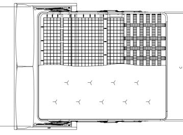
A – Steel structure dimensions 166/180cm B – Slatted base frame dimensions 195×150/164cm
