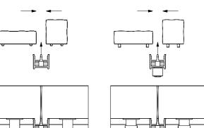
Hooks for assembly for indoor elements with Hooks for assembly for outdoor elements with
